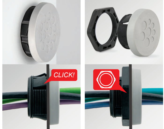
Mounting type 1: Snap into the cut-out For wall thickness 1 – 2.5 mm
